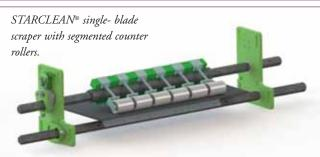
single blade scrapers cannot adapt to the belt properly and therefore the cleaning result is more than limited, Schulte Strathaus uses an assembly with segmented rollers at the inside of the belt, which gently adapts the belt to the cleaner. With this new system, even the stickiest materials can be perfectly scraped off the belt, without material buildup on the scraper. The roller assembly is equipped with the proven quick tensioning device for easy tensioning.
